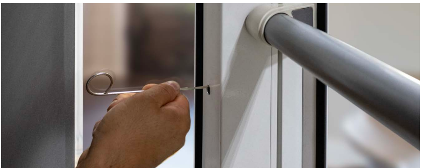
Figure 14: Inside access to emergency opening
