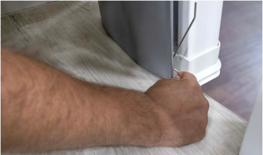
Figure 13: Emergency key behind inside panel
